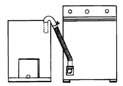
If a longer drain hose is needed, drain hose (Part No. 388423) and hose extension kit (Part No. 285442) are available from authorized parts distributors. If drain hose must be shortened, use hose kit (Part No. 285442).
